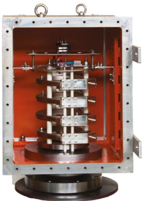
Slip ring collector for potentially explosive areas, designed to transfer current from a fixed supply point to a rotating structure, transmitting power and control signals, both analogue and digital, to mobile units. Thanks to the high degree of customization, it is used in a variety of industrial sectors where risk of explosion is feasible (Zone 1 and 2).
