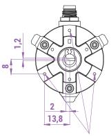
Ø holes 1.8 mm ↓ hole depth 8 mm No.3 screws ISO7049-ST2.5
