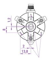
Ø holes 1.8 mm Thole depth 8 mm No.3 screws ISO7049-ST2.5
