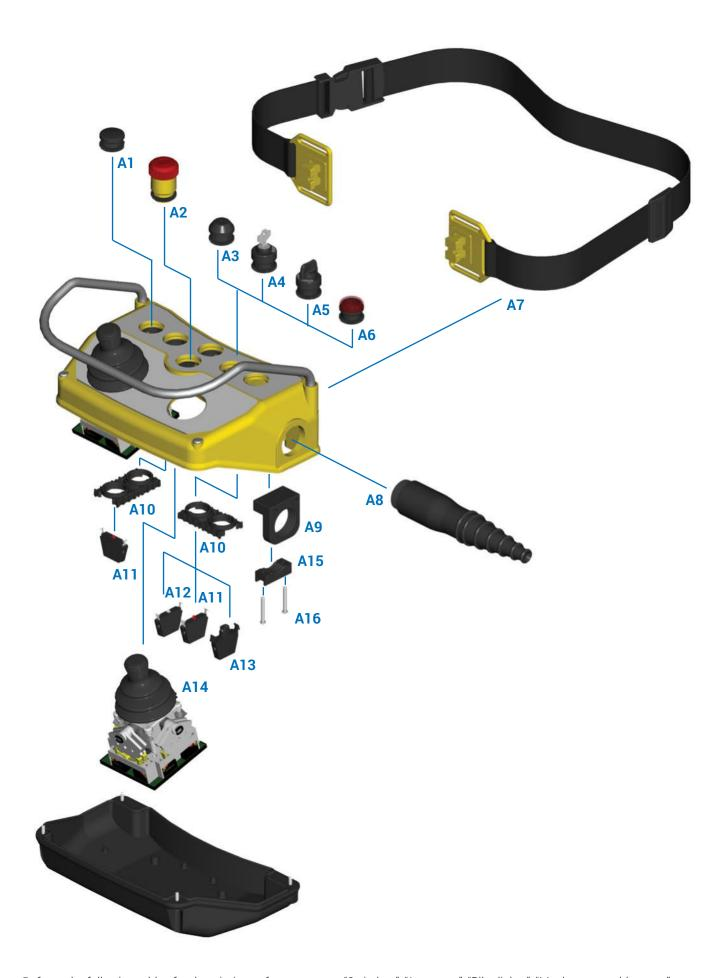
Refer to the following tables for descriptions of components: "Switches", "Actuators", "Pilot lights", "Mushroom pushbuttons", "Selector switches", "Joysticks" and "Accessories".
