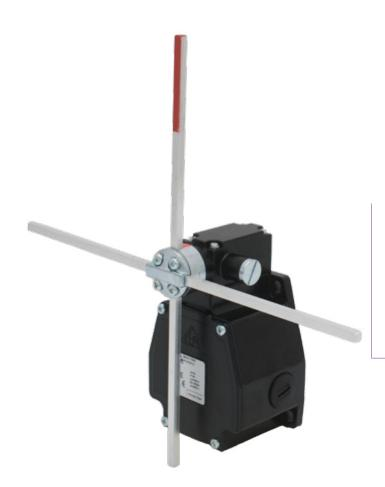
Multiple position limit switch, also suitable to be used as a low resolution absolute encoder, designed to control the movement of overhead travelling cranes, hoists and complex machine tools.
