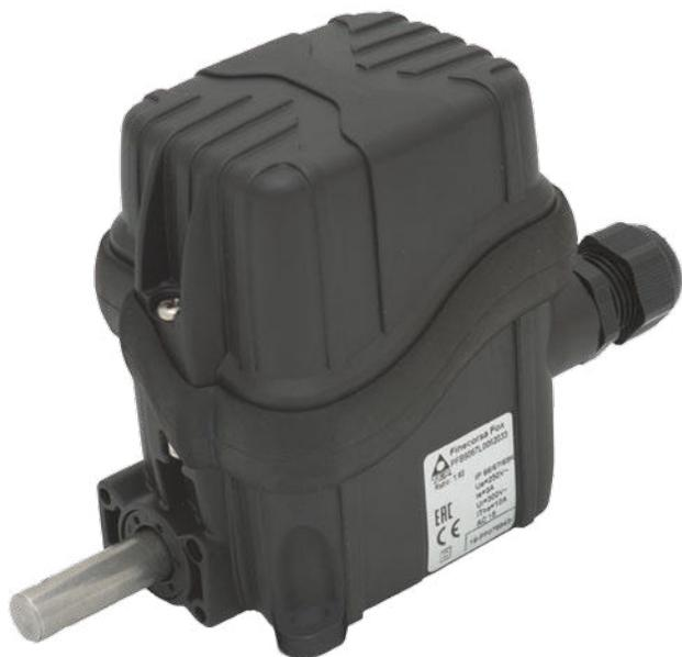
Rotary limit switch used to control and measure the movement of industrial machines by reading the rotation angle and/or the number of revolutions of a shaft. Fox is used on wind turbines to control the position of the nacelle or the pitch angle of the blades.
